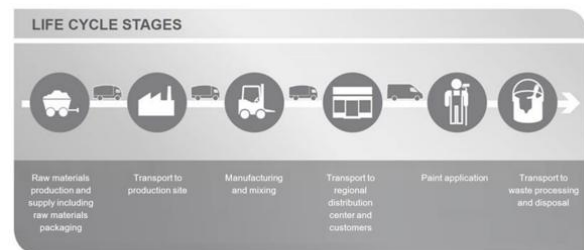
Figure: LCA process diagram according to EN 15804 (7.2.1)
