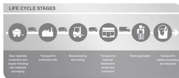
Figure: LCA process diagram according to EN 15804 (7.2.1)
